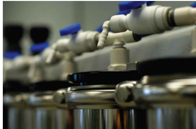
Membrane test ports for isolation pro ling
